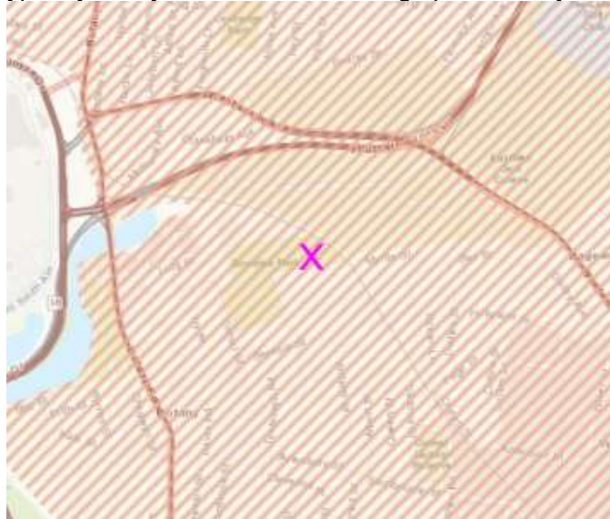
Figure 15 Extract from Appendix A – Botany Bay Sand Aquifer, showing areas in orange hatching whereby absorption is preferred over onsite detention (Source: SM Technical Specification)
